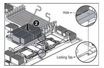
11 Push down the heat sink retaining levers (3) and lock them under the retaining hooks on the heat sink socket.
